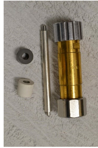
Figure 2: Left: WG16 waveguide spacer and specimens. Right: 14-mm coaxial line and specimens.
