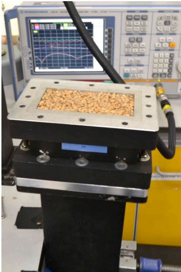
Figure 1: Measurements on a granular material in waveguide size WG8 (1.7 GHz to 2.6 GHz). The top waveguide adaptor has been disconnected for the photo.
