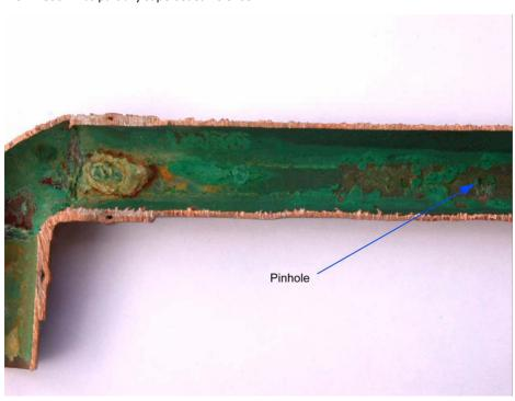
**Figure 3.** Pinhole caused by flux attack. 5
