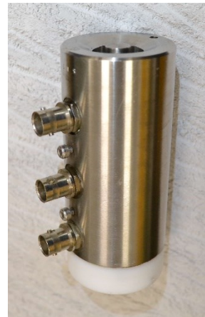
Figure 1: Three-terminal admittance cells for measurement of permittivity and loss. Left: schematic of the cell used to measure laminar solid specimens [2]. The 'low' terminal is 38 mm diameter. Right: NPL liquid cell.
