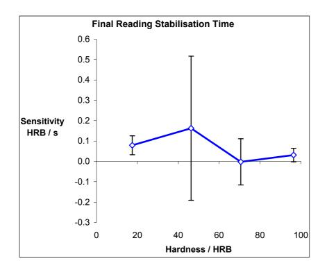
The following graph shows the sensitivity of the HRB scale to indenter velocity, as measured at NIST.
